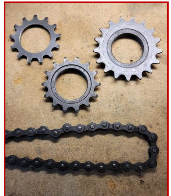
My 40 year old track chain and cogs. The chain is thick, strong as heck. But would those 13, 14, and 17 tooth cogs be the right gearing with a 39 tooth chainring?
